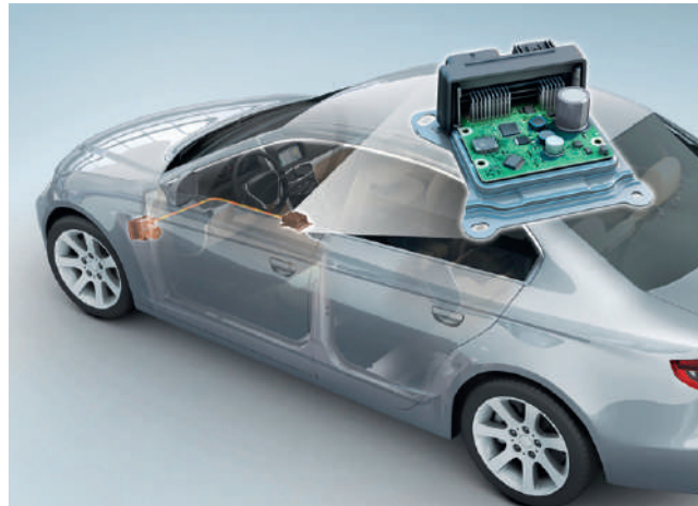
Figure 4.119 Electronic control unit control of the brakes
